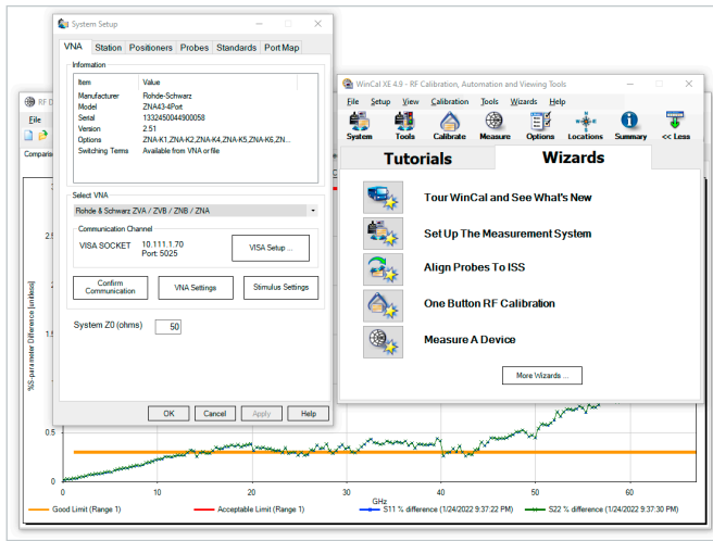
R&S®ZNA43 selected as VNA in FormFactor WinCal XE software.
