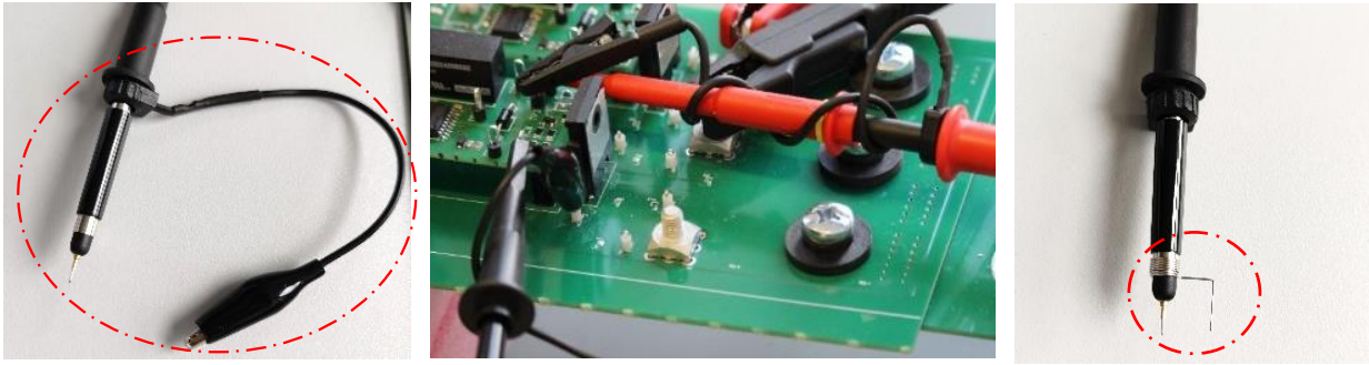
Figure 16: DPT voltage measurement with passive probes with large loop(left) and counter measures (center) and (right)
