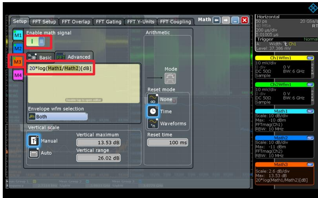
Fig. 3-6: Formula for the amplitude difference of RX 1 and RX 2
