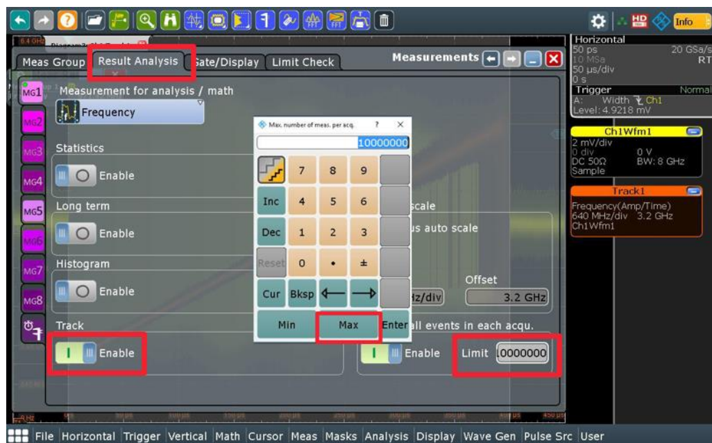
Fig. 2-12: Settings for the chirp measurement (frequency versus time)
