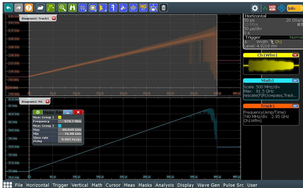
Fig. 2-15: Diagram1 (blue trace) shows the low pass filtered demodulated chirp signal in time domain beginning at 77 GHz
