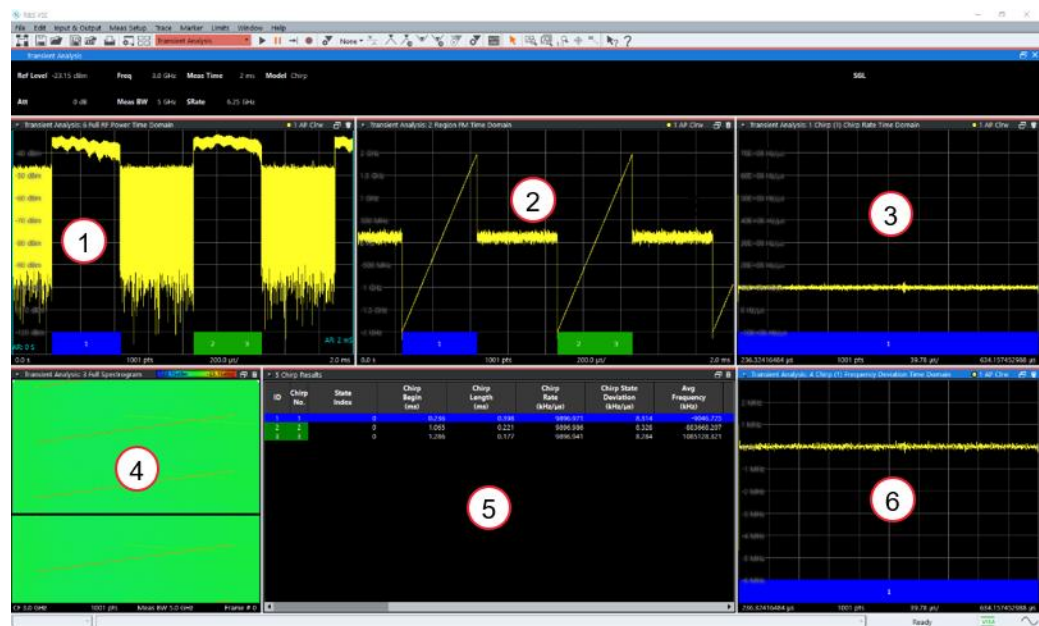
Fig. 2-20: Chirp analysis with the VSE software
