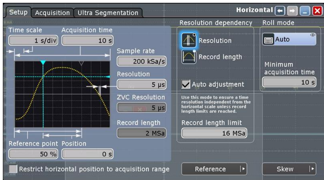
Figure 4-2: Data Acquisition Setup on the RTO
