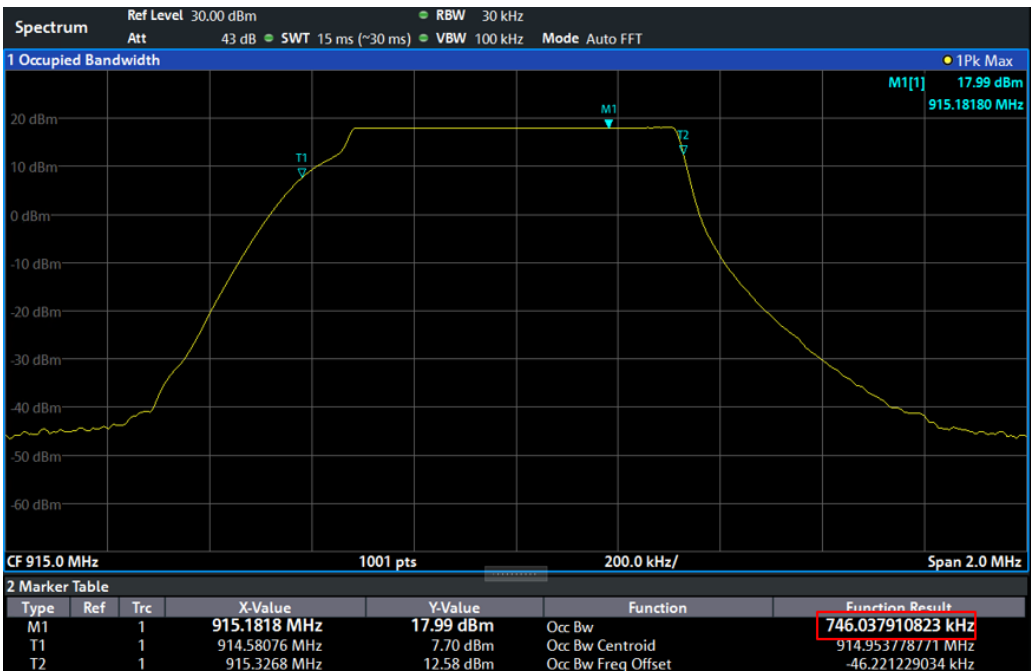
Figure 2-5: Measurement of OBW with SF = 12
