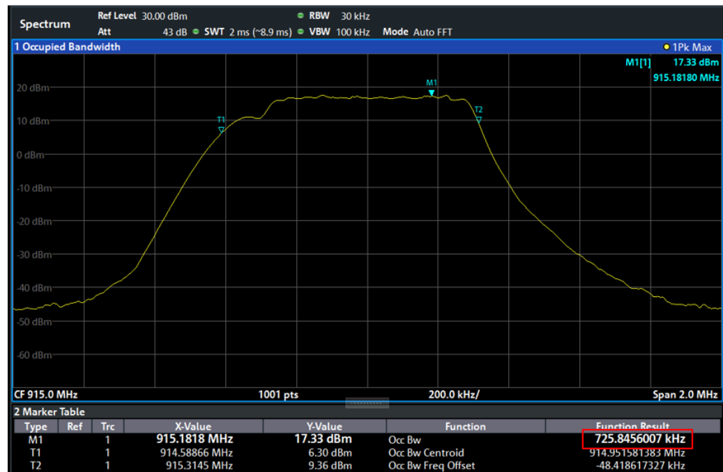
Figure 2-4: Measurement of OBW with SF = 7
