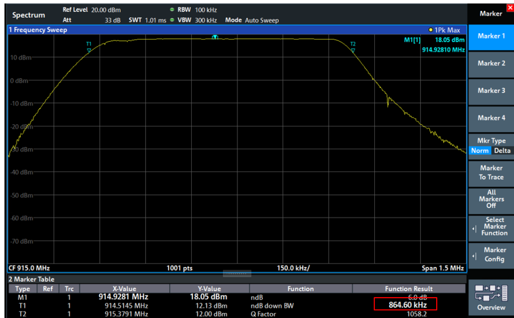
Figure 2-3: Measurement of 6 dB bandwidth with SF = 12
