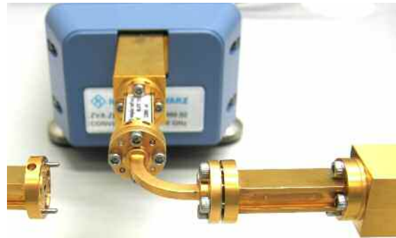
Fig. 4.8b: Unknown Through standard between waveguide test ports 2 and 4
