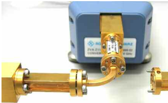
Fig. 4.8a: Unknown Through standard between waveguide test ports 1 and 4
