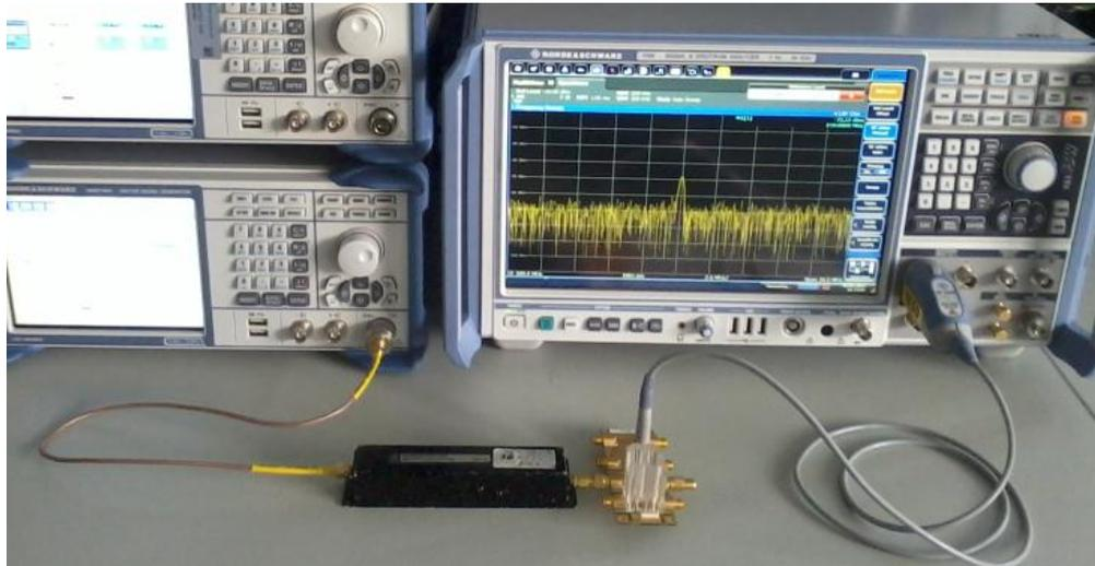
Fig. 3-5: Test setup for harmonic distortion test for RT-ZS30at 100 MHz
