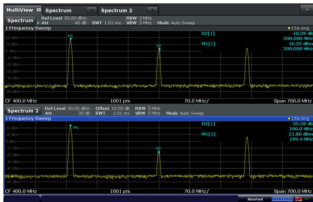
Fig. 4-2: Test result of the differential amplifier connected to the spectrum analyzer
