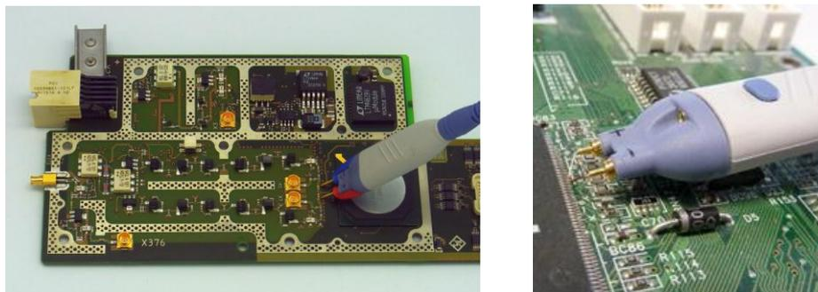
Fig. 2-7: Examples for a differential probe directly connected to a circuit
