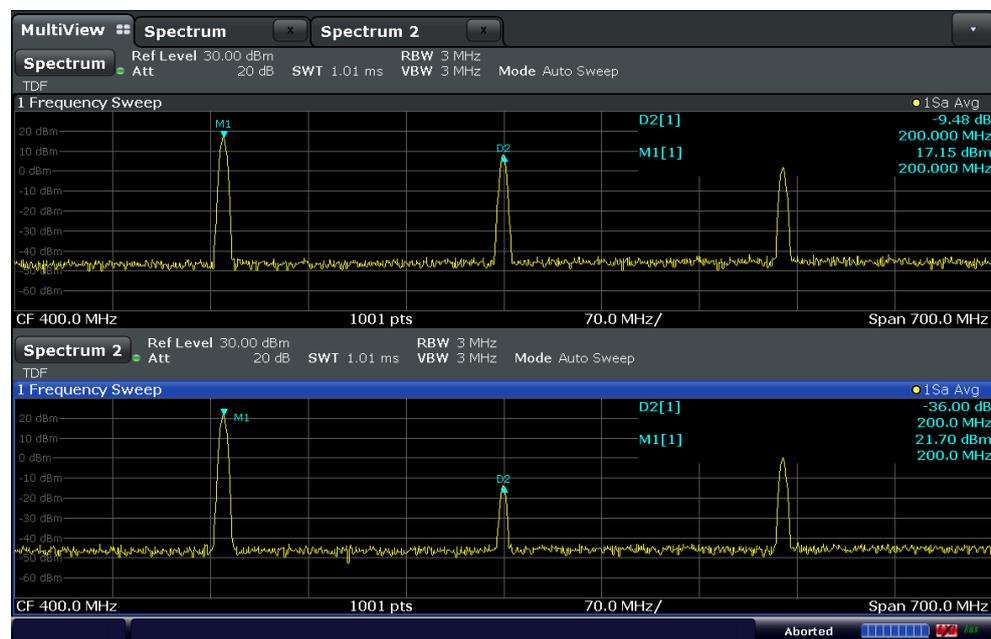
Fig. 4-4: Test result of the differential amplifier connected to the spectrum analyzer
