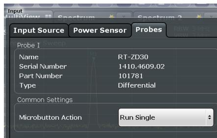
Fig. 2-5: RF input and Probe configuration on the R&S FSW spectrum analyzer
