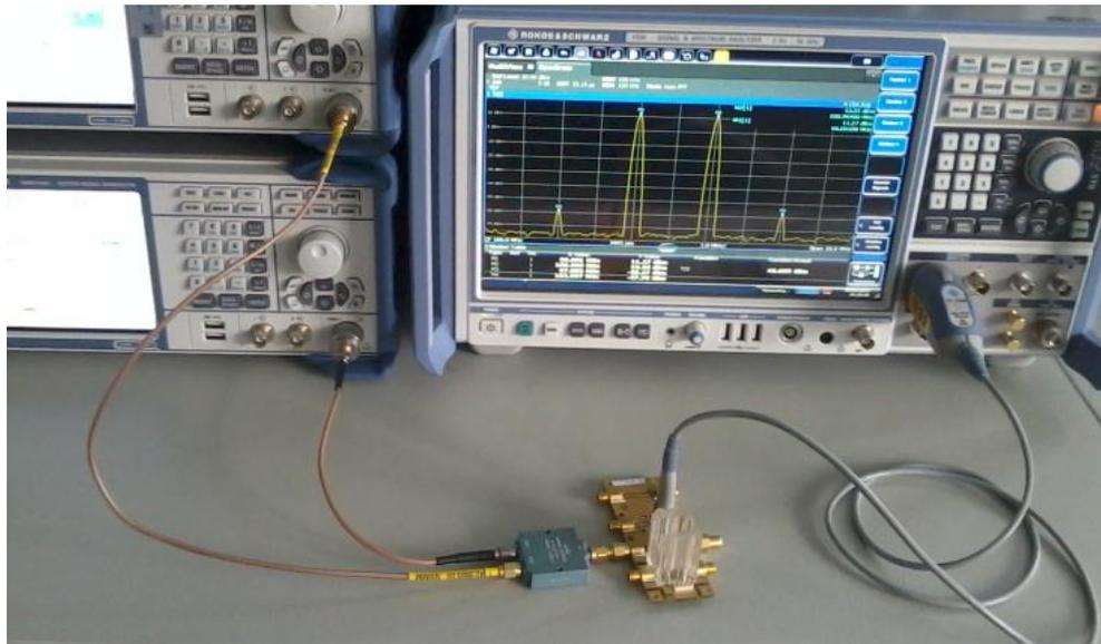
Fig. 3-3: Test setup for intermodulation distortion test of the RT-ZS30 at 500 MHz
