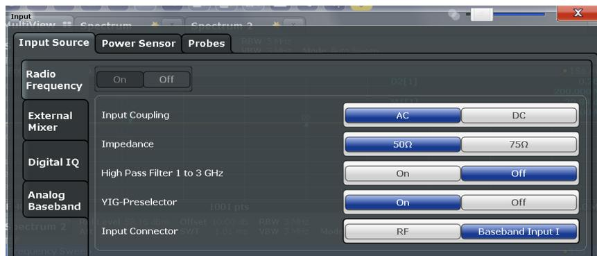
Fig. 2-6: RF input selection dialog on the R&S FSW spectrum analyzer
