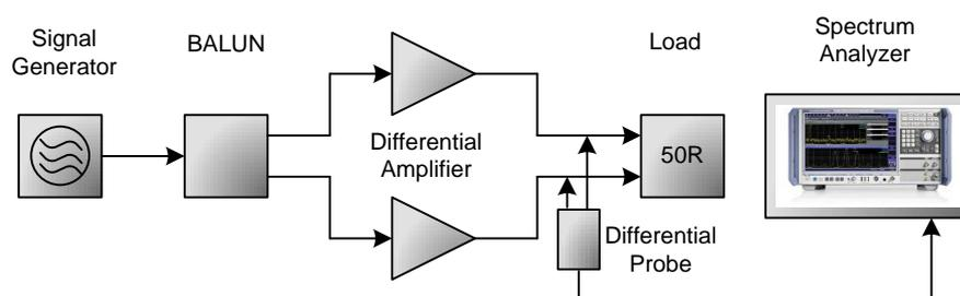
Fig. 4-1: Block circuit of the differential amplifier test setup
