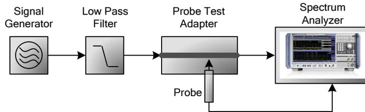
Fig. 3-4: Block circuit of harmonic distortion test setup
